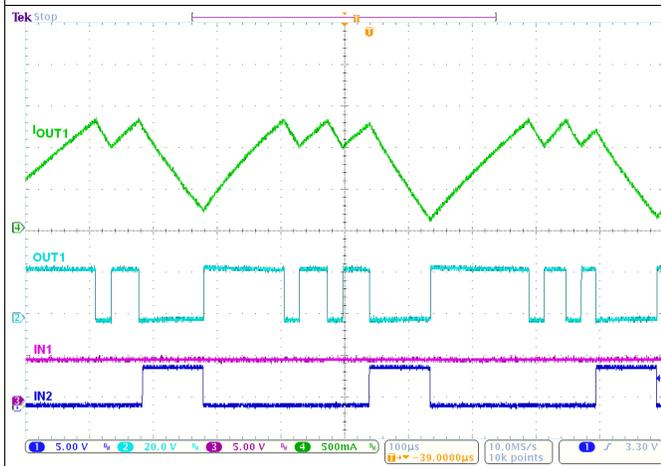
Figure 12. Current Regulation With  $R_{SENSE} = 0.26 \Omega$
