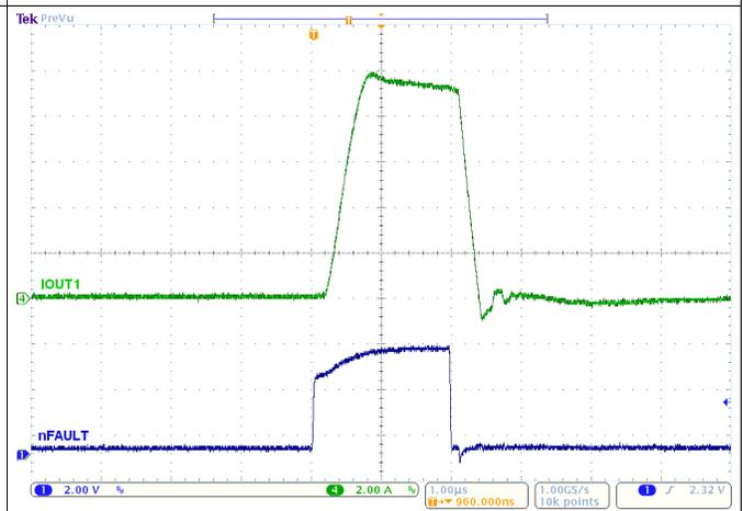
Figure 13. OCP With 24 V and Outputs Shorted Together
